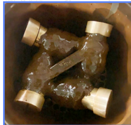
Magnetite collected on the external surface of the Rare Earth Magnetic Grate
